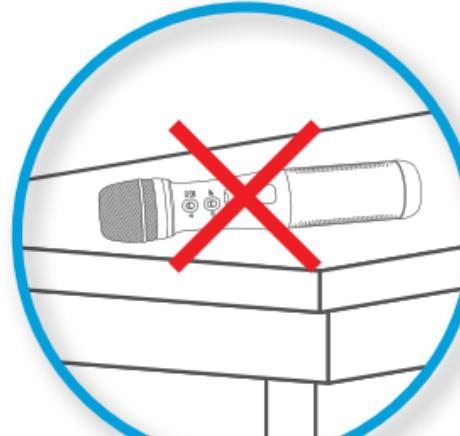
To avoid feedback (squealing noise) do not set the unit on a table or hard surface when it is turned on.
